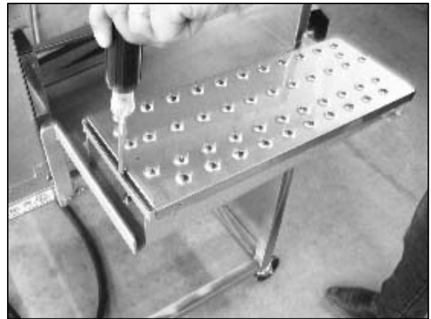
26. Insert flat tip screwdriver into finger assembly if it cannot be removed by hand.
